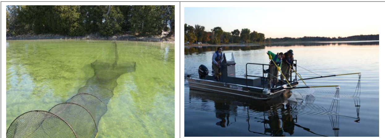
Photograph 3.6-1. Fyke net positioned in the littoral zone of a Wisconsin Lake (left) and an electroshocking boat (right).
